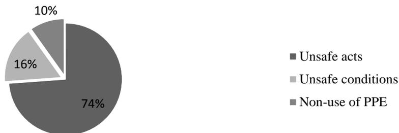
**Figure 2.** Relative frequency distribution of the main causes of incidents at Yazd combined cycle power plant
