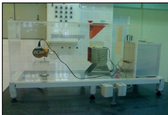
Figure 1. Photograph of airborne pollutant simulation chamber
